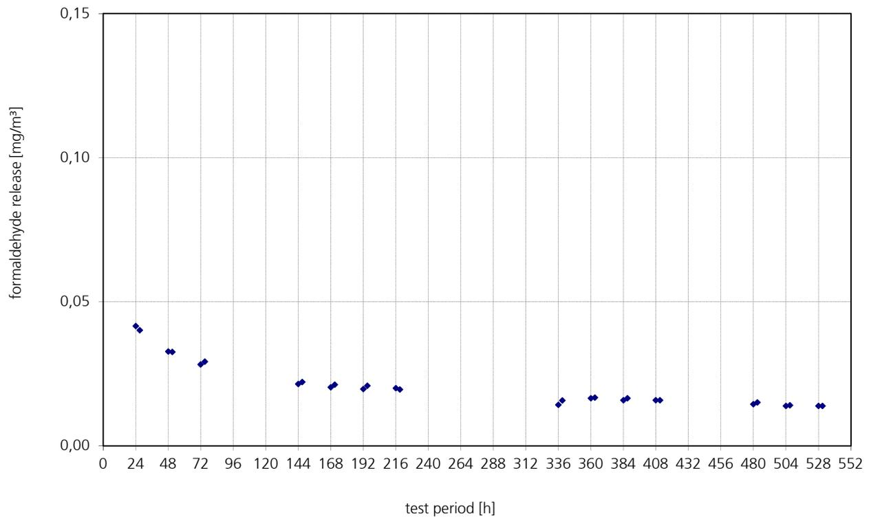
Figure 1: Course of formaldehyde release [mg/m<sup>3</sup>] in the test chamber during the measurement of an item named "SWP 27 (9-9-9) mm Spruce – Thickness: 27 mm" sent by AGROP NOVA a.s. in 79843 Ptení (Czech Republic)
